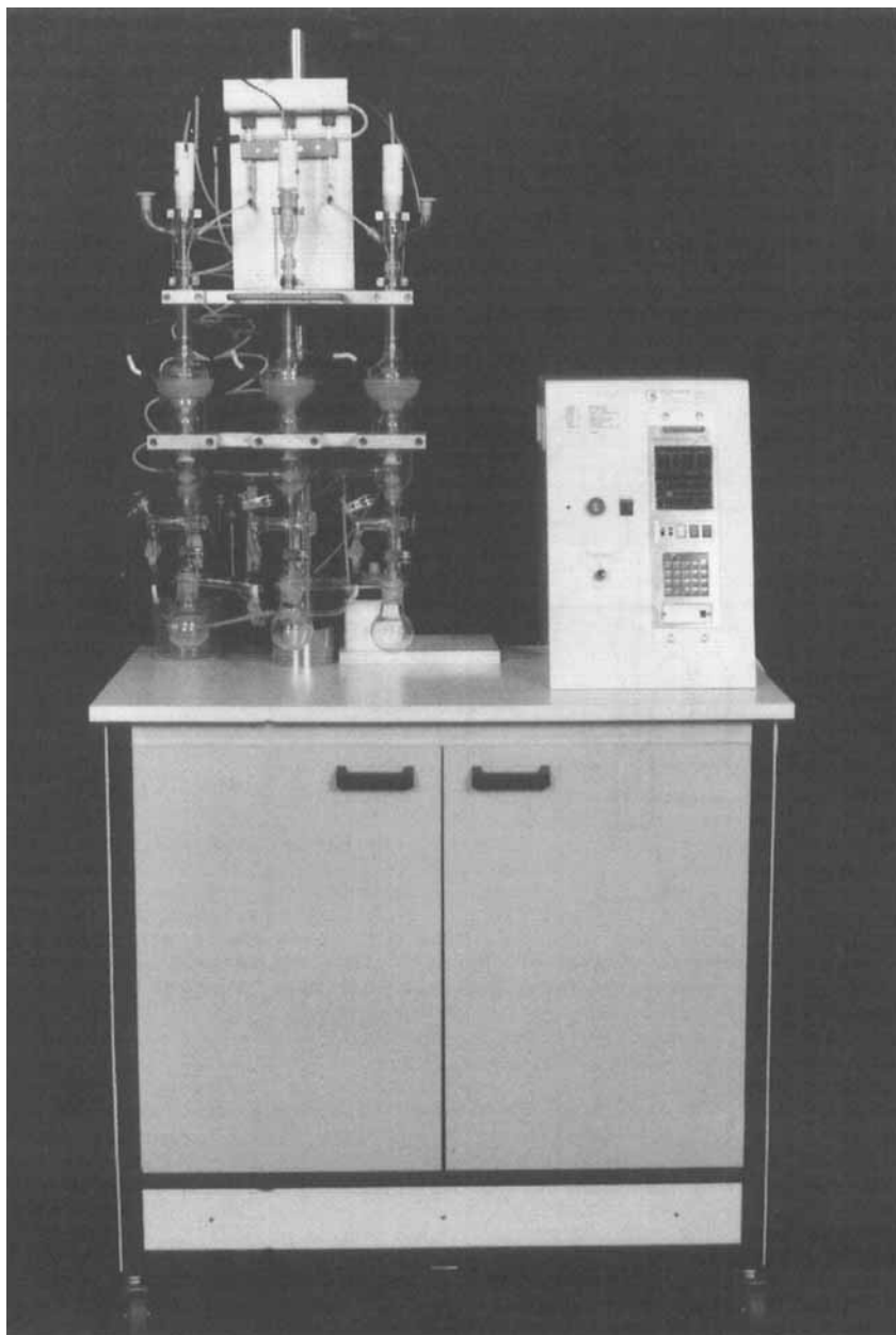
Fig. 2 Electronically-controlled extraction apparatus according to Amin and Korbakis.
